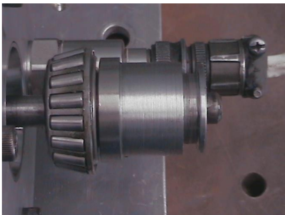
Figure 37: Test bearing inner race bushing assembly
