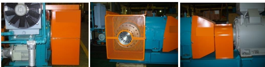
Figure 59: A typical gearbox from our industrial partner, showing the output- and input shafts' protective shrouds
