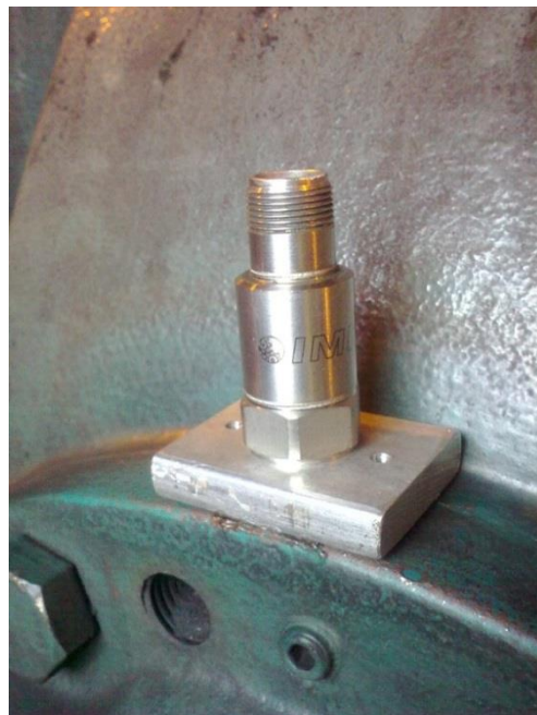
Figure 58: Detail showing accelerometer mounting
