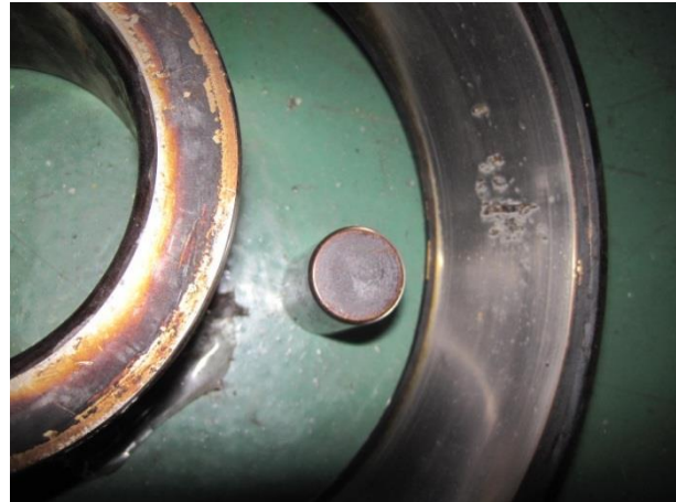
Figure 77: Inspected bearing with damage
