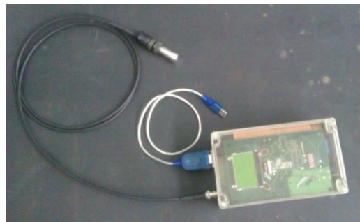
Figure 17: Illustration of the Beta prototype with accelerometer and RS232 cable connected
