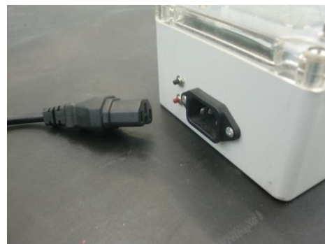
Figure 18: Battery socket and power cord of the Beta prototype
